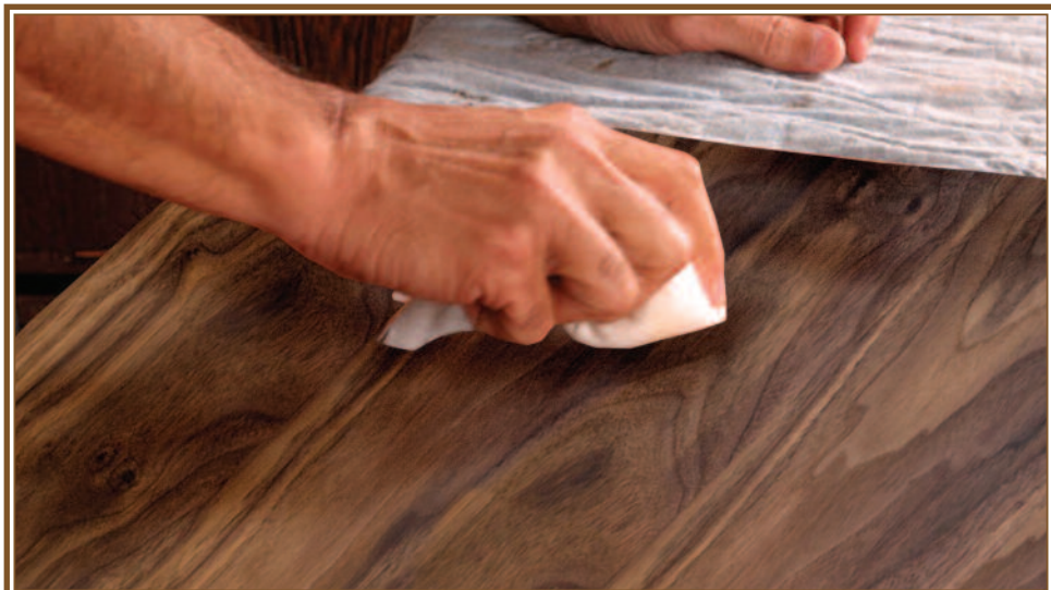
Applying the French polish with a 'loaded' rubber
